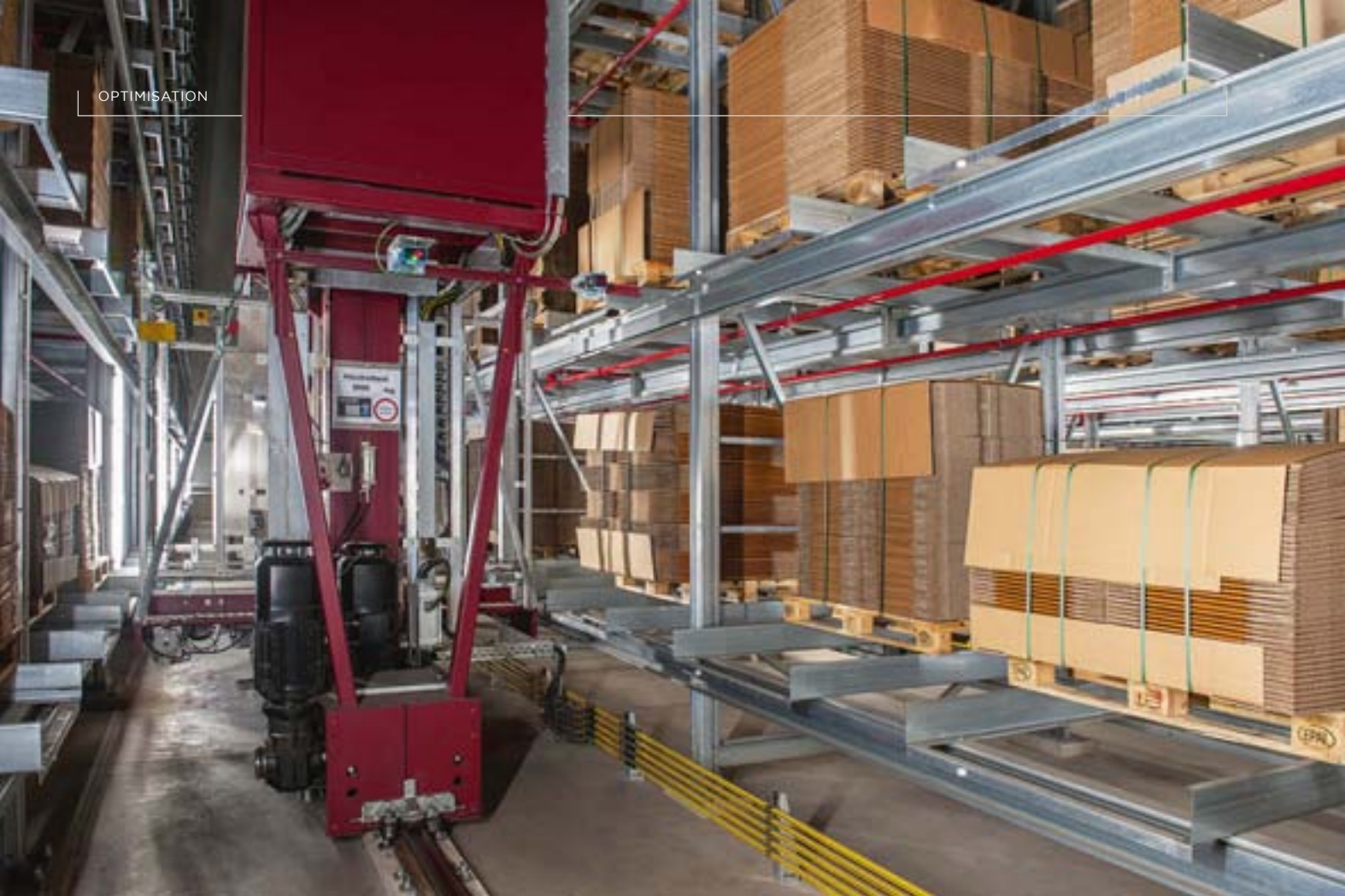
View into the SRM aisle with multi-deep storage of different pallet formats.
