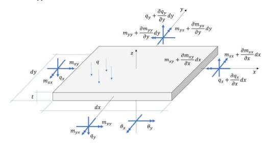
Figure 1. Plate stress resultants and rotations.
