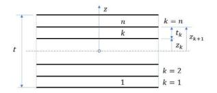
Figure 4. Laminate material of thickness *t* with *n* orthotropic homogeneous layers.
