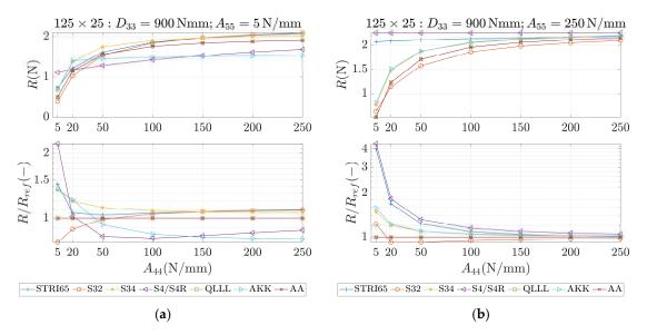
**Figure 11.** Reactions (first row) and reactions to the reference (analytical) solution (second row) for  $125 \times 25$  sample,  $D_{33} = 900$  Nmm and different values of  $A_{44}$ . (**a**)  $A_{55} = 5$  N/mm and (**b**)  $A_{55} = 250$  N/mm.
