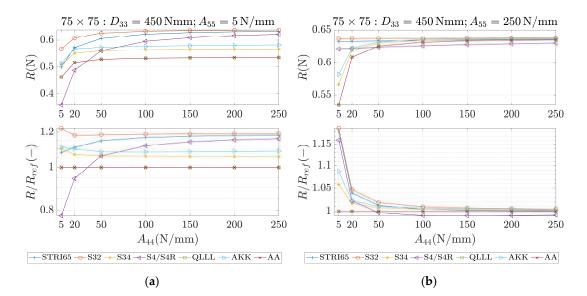
**Figure 7.** Reactions (first row) and reactions to the reference (analytical) solution (second row) for 75 × 75 sample,  $D_{33} = 450$  Nmm and different values of  $A_{44}$ . (a)  $A_{55} = 5$  N/mm and (b)  $A_{55} = 250$  N/mm.
