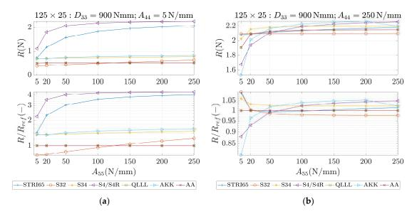
**Figure 12.** Reactions (first row) and reactions to the reference (analytical) solution (second row) for 125 × 25 sample,  $D_{33} = 900$  Nmm and different values of  $A_{55}$ . (**a**)  $A_{44} = 5$  N/mm and (**b**)  $A_{44} = 250$  N/mm.
