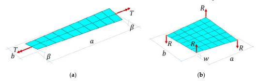
**Figure 2.** Two mechanical test setups to measure transversal shear stiffness of the sample: (**a**) via torque and angle of rotation and (**b**) via pair of force and vertical displacement (plate torsion test).
