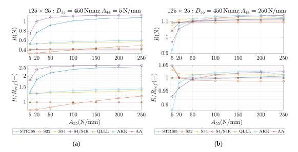
**Figure 10.** Reactions (first row) and reactions to the reference (analytical) solution (second row) for  $125 \times 25$  sample,  $D_{33} = 450$  Nmm and different values of  $A_{55}$ . (a)  $A_{44} = 5$  N/mm and (b)  $A_{44} = 250$  N/mm.
