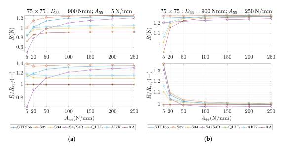
**Figure 8.** Reactions (first row) and reactions to the reference (analytical) solution (second row) for 75 × 75 sample,  $D_{33} = 900$  Nmm and different values of  $A_{44}$ . (**a**)  $A_{55} = 5$  N/mm and (**b**)  $A_{55} = 250$  N/mm.
