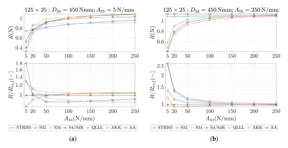
**Figure 9.** Reactions (first row) and reactions to the reference (analytical) solution (second row) for 125 × 25 sample,  $D_{33} = 450$  Nmm and different values of  $A_{44}$ . (a)  $A_{55} = 5$  N/mm and (b)  $A_{55} = 250$  N/mm.
