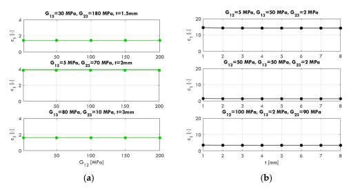
**Figure 4.** Influence of  $G_{12}$  (a) and effective thickness t (b) on the value of the  $c_1$  parameter.
