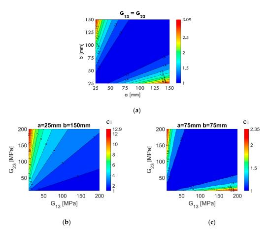
**Figure 5.** Influence of the relation a/b (**a**) and  $G_{13}/G_{23}$  for a sample of  $25 \times 150$  mm (**b**), and a sample of  $75 \times 75$  mm (**c**), on the value of the  $c_1$  parameter.
