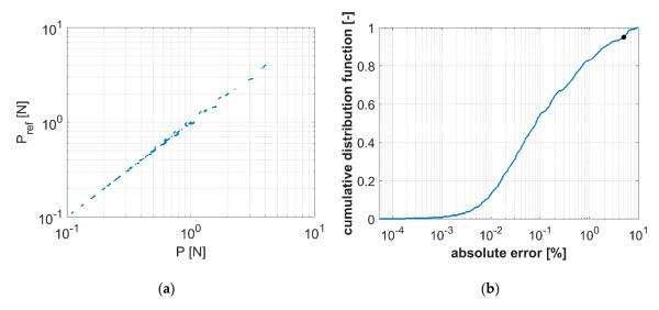
**Figure 6.** Solution error for P from the modified analytical approach, and  $P_{ref}$ , the reference values derived from the FEM: (a) logarithmic regression plot of raw data and (b) cumulative distribution function plot of the data.
