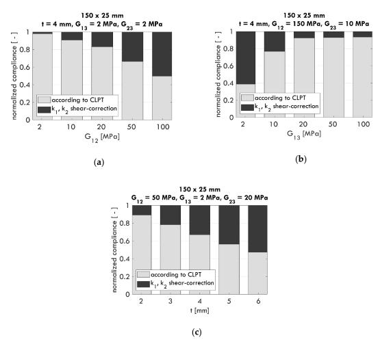
**Figure 2.** Examples of significant influence of transverse shear on sample compliance for selected values of  $G_{12}$ ,  $G_{13}$ ,  $G_{23}$ , and t with respect to changing values of  $G_{12}$  (**a**),  $G_{13}$  (**b**), and t (**c**).
